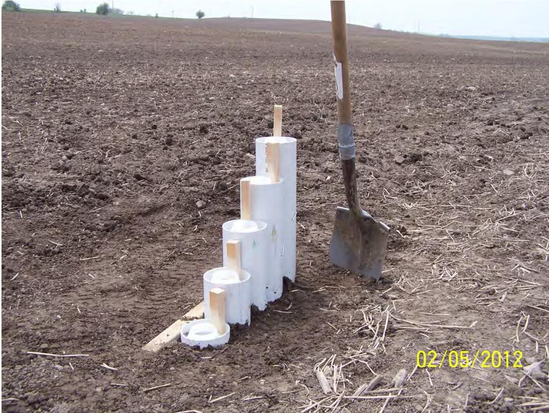
**Plate 1:** Pipe organ sampler designed to capture runoff waters at different heights above the ground surface (from left to right: 0, 5, 10, 15, and 20 centimetres).
