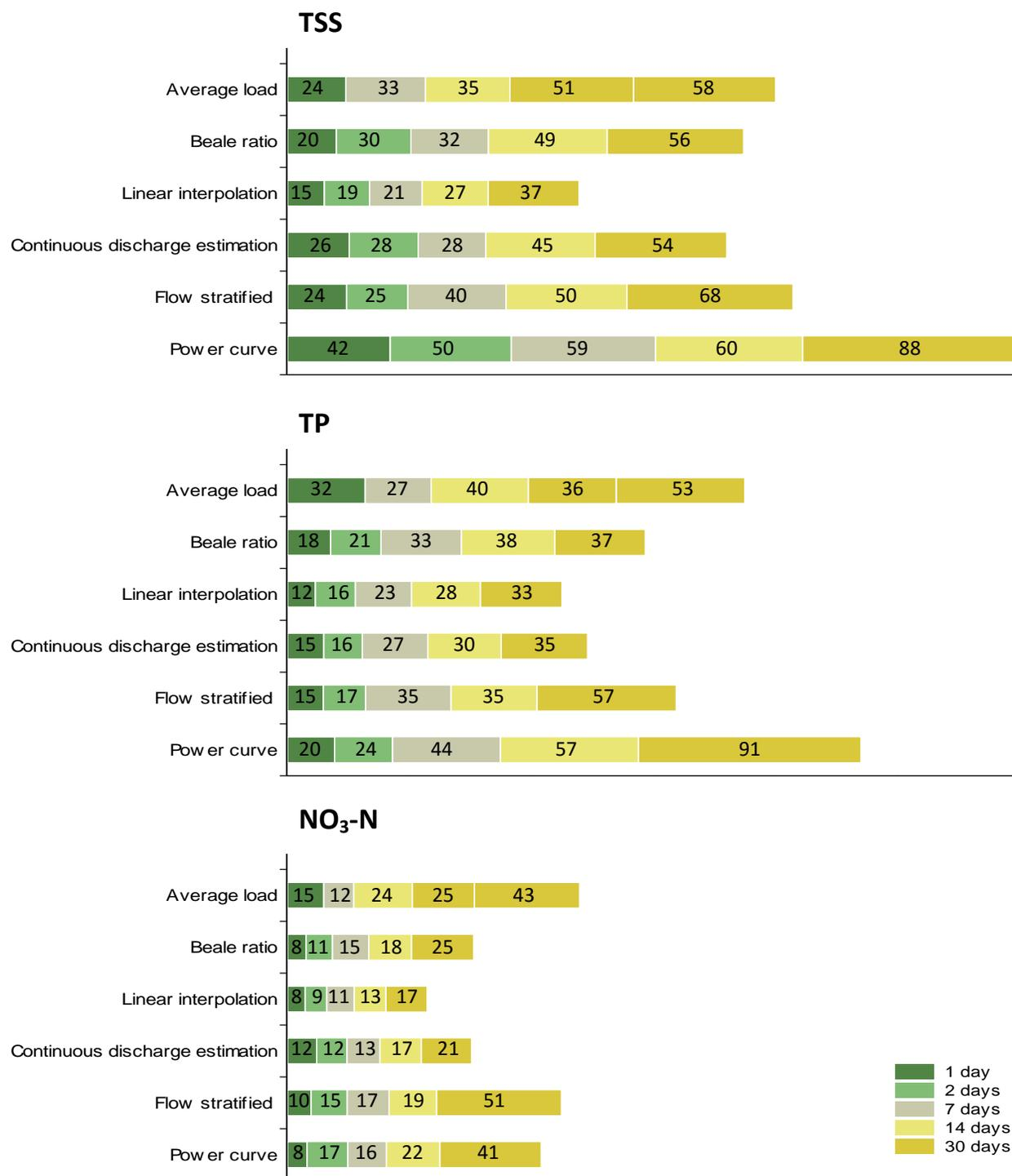
**Figure 2:** Root mean squared error (%) for six load estimation algorithms over five different sampling frequencies. Values shown are the mean difference between the reference (“true”) loads and the estimated loads using water quality data from Gully Creek, Garvey Creek/Glenn Drain, and Trick’s Creek.
