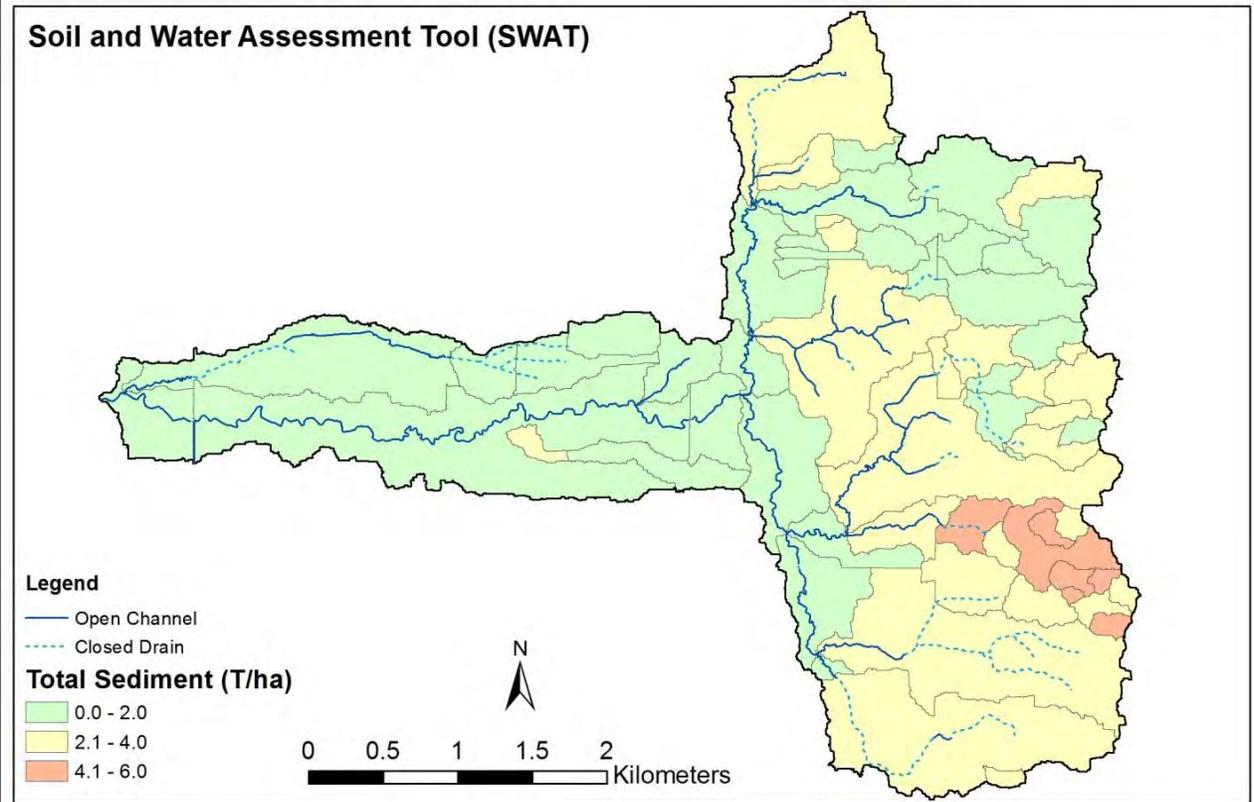
**Figure 4:** Sediment loadings per catchment in Gully Creek watershed as calculated by PTMApp and SWAT
