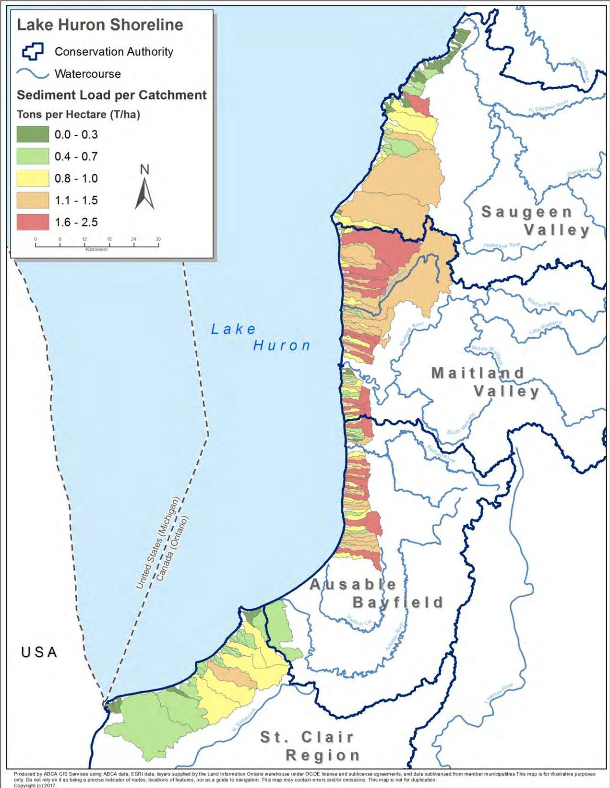
Figure 6: PTMAApp results along the shoreline for sediment loading (represented as T/ha per catchment)
