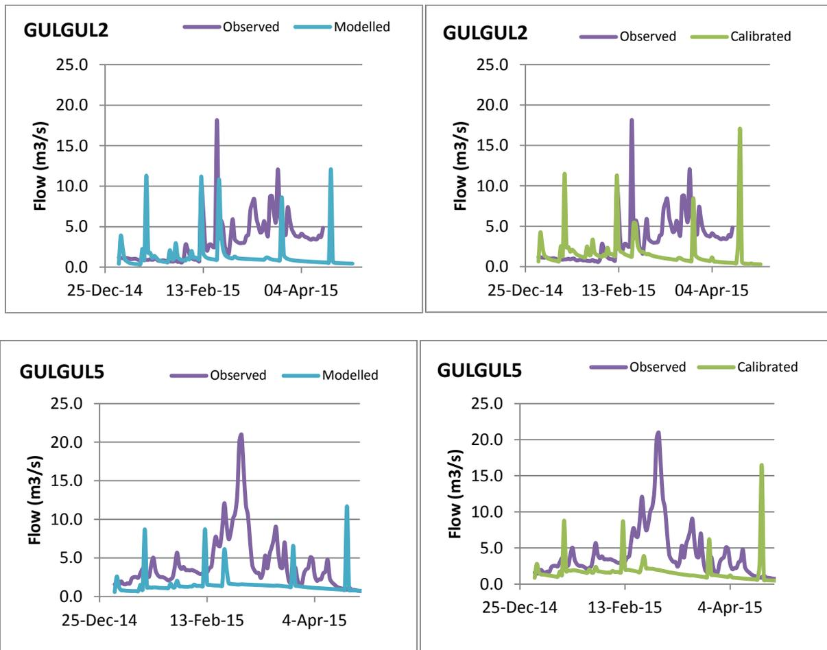
**Figure 3:** SWAT simulated flow versus observed flow at GULGUL2 and GULGUL5 (blue – modelled with default parameters, green – modelled with calibrated parameters and purple – observed flow)
