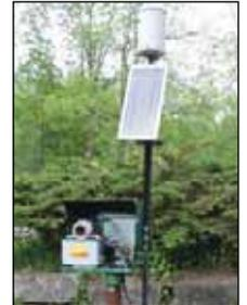
ABCA upgraded water-level telemetry (automatic measurement and transmission of data from remote sites) at some wells in 2015.
