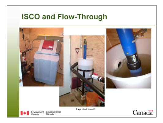
In the hut, we use a flow-through system. River water is continuously pumped up to the hut via a line wrapped with heat trace wiring to prevent freezing. The ISCO automated water quality sampler samples from the line as per its program. The water flows through an in-line reservoir, into which a YSI sonde collects real-time measurements of conductivity and other parameters.
