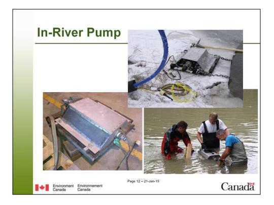
After much investigation, we determined to use in-river pumps to deliver a continuous flow to huts that are installed adjacent to the rivers, from which we collect samples for water quality. These pumps need to be strong enough to deliver water into the hut, need to not become plugged by debris, and need to withstand very high flows (up to 800 m3/s!) that can scour the river beds. We need to be able to flush the pumps also in order to prevent blockages.
