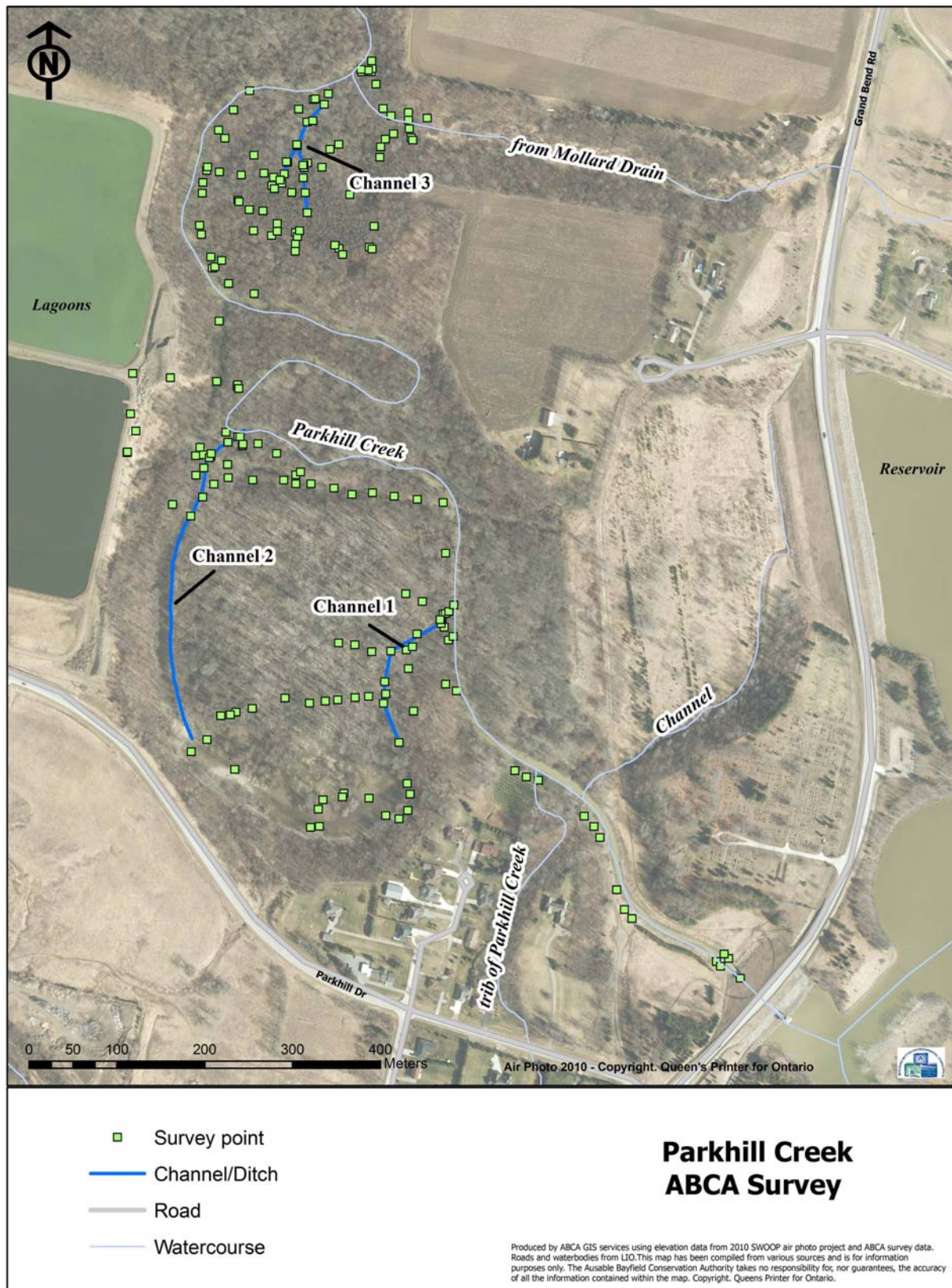
Figure 4: Parkhill Creek wetland survey indicating watercourses, dug channels and survey points within the area of focus.
