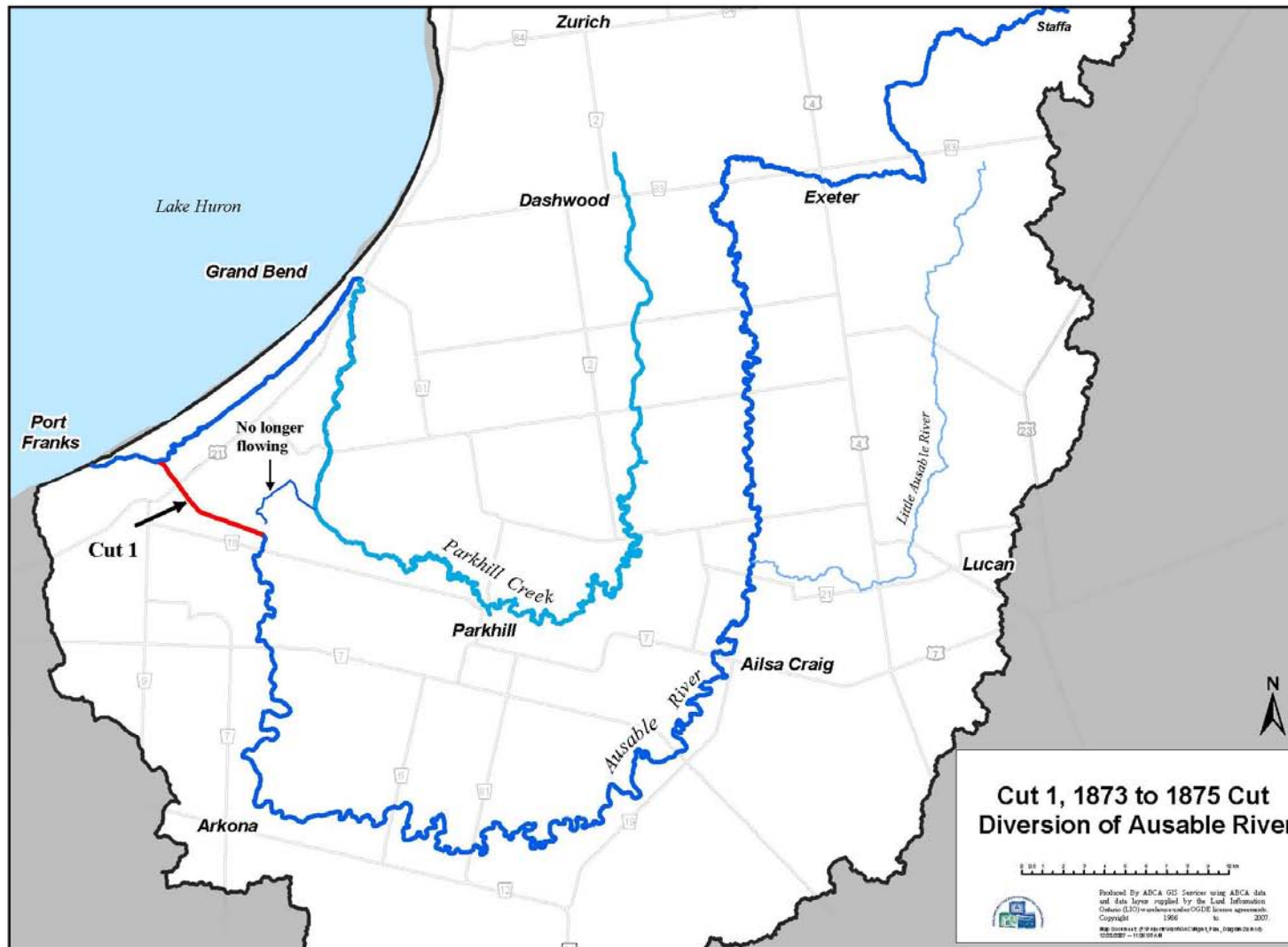
Figure 3: Configuration of the Ausable River after the diversion in 1873 to 1875
