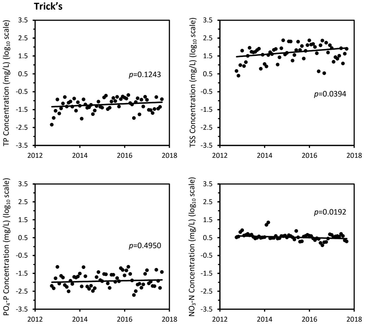
**Figure E-5: Water quality trends in monthly flow-weighted mean concentrations for Trick's Creek (October 2012 to September 2017).**
