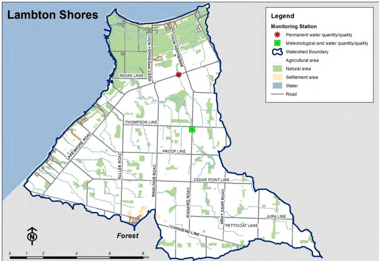
Figure A-5: Location of the water quantity/quality monitoring station (red) in Shashawandah Creek.
