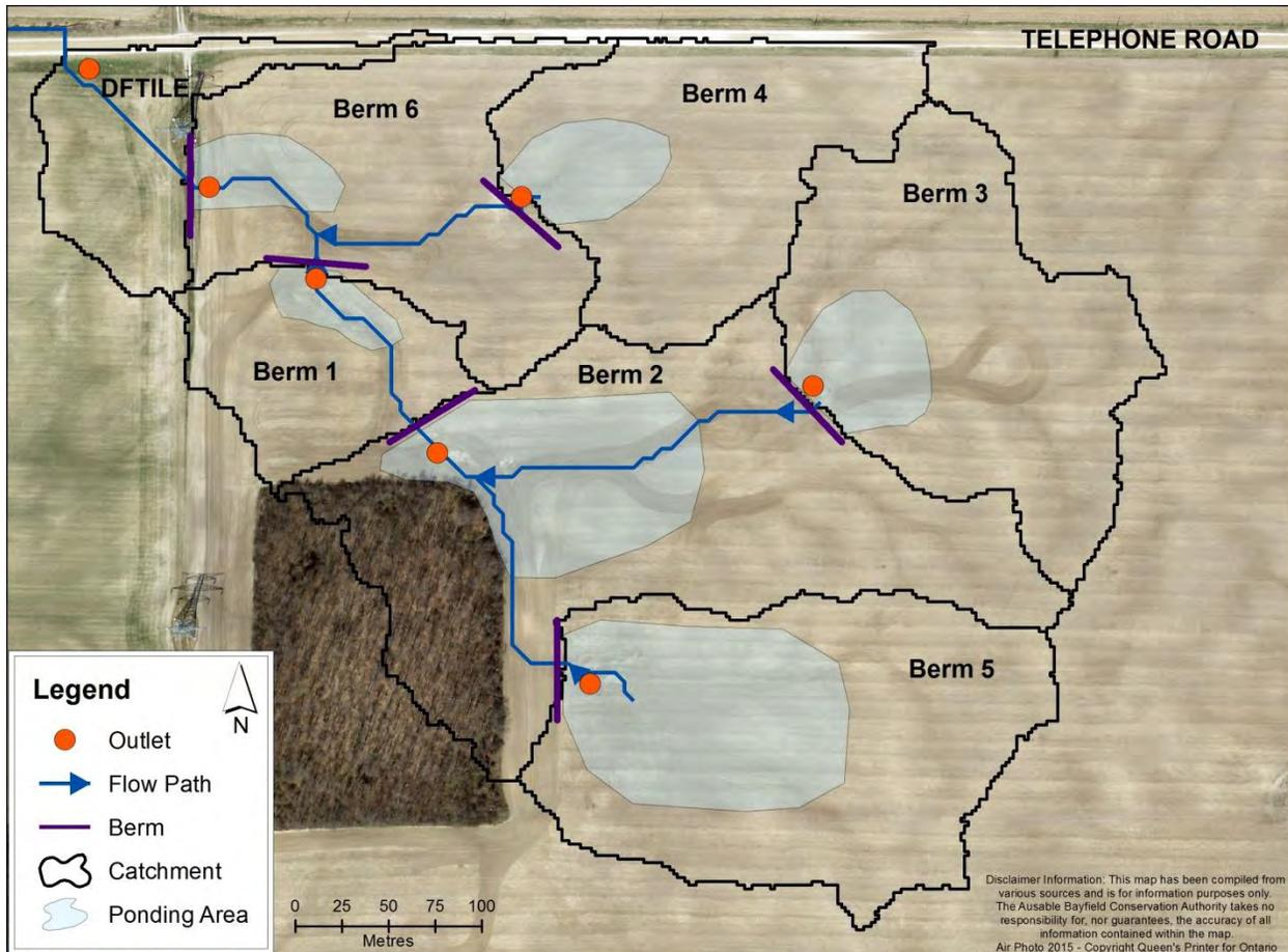
**Figure 9: Map of a monitored field in the Gully Creek watershed. Only WASCobS 2, 3, 5, and the tile (top left) are monitored for water quantity and quality. Flow direction is indicated by blue arrows.**
