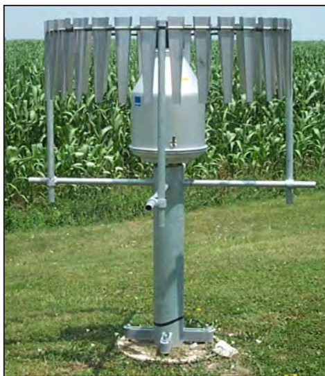
A GEONOR weighing gauge precipitation station was installed at the ABCA Administration Centre in Exeter.
