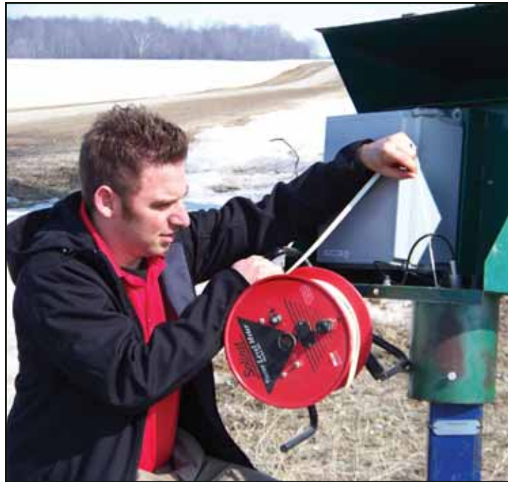
ABCA lands and water technologist Davin Heinbuck checks one of 14 active monitoring wells in Ausable Bayfield watersheds.
