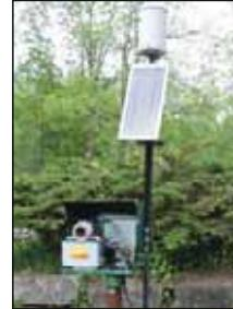
ABC upgraded water-level telemetry (automatic measurement and transmission of data from remote sites) at some wells in 2015.
