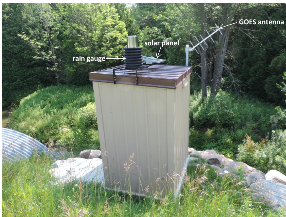
Figure 3: A stream gauging station with a tipping bucket rain gauge, solar panel, and Geostationary Operational Environmental Satellite (GOES) antenna.
