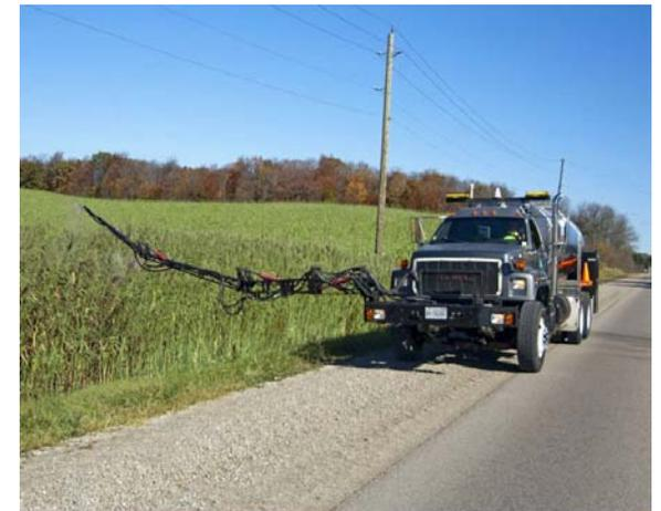
Boom sprayer used to control roadside invasive *Phragmites*
