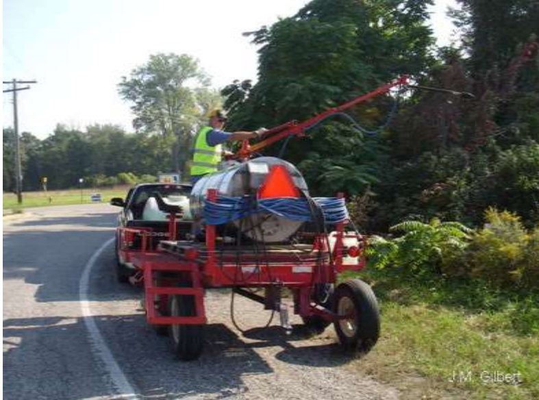
Figure 13. Frank Letourneau (Dover Agri-Serve) using a boom sprayer to control invasive Phragmites along a road in Chatham-Kent.
