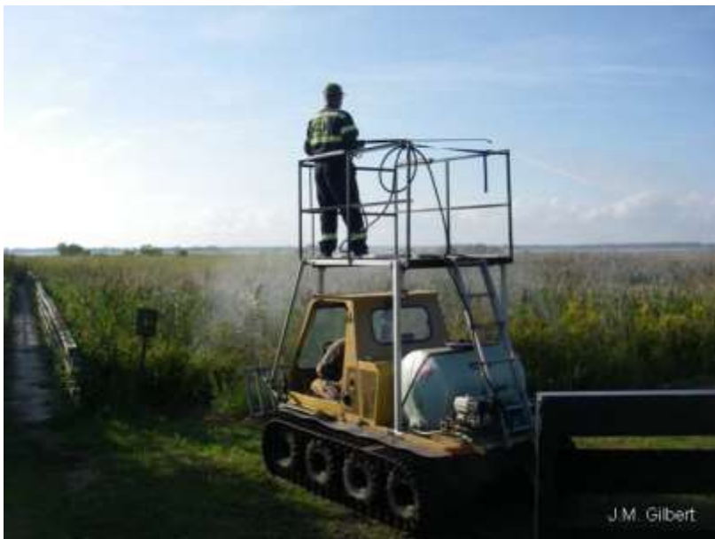
Figure 14. Frank Letourneau (Dover Agri-Serve) using a retrofitted Centaur™ to control invasive Phragmites located within difficult-to-access terrain.
